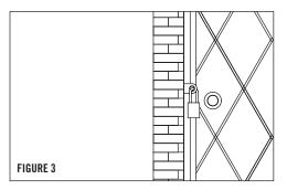
NOTE: Door gates can be installed in the casing of the door or outside the door. Gate can be mounted on the left or right. Simply turn the gate upside down to mount on the opposite side.
